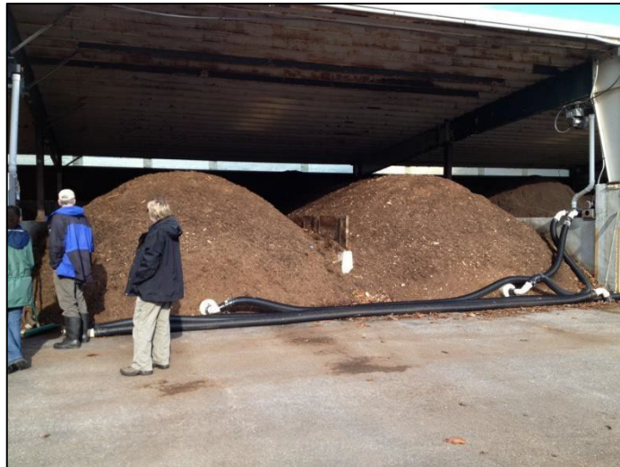
Little River Compost Facility (Lisbon)-Aerated Static Piles (photo by Mark King)
