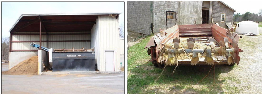
Mixing Equipment commonly used for composting. Image on left is of Kuhn Knight™- Reel Auggie 3130 Mixer. The image on the right is of a typical manure spreader found on nearly any farm. (photos by Mark King)
